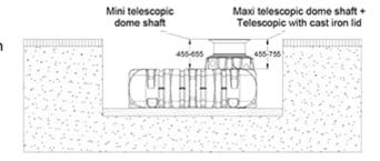
Maximum coverage heights with extension and telescopic dome shaft.
