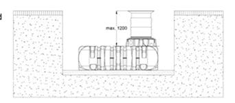
Cover heights with cast iron telescopic dome shaft (class B) in area driven over by vehicles up to 3.5 tonnes.
