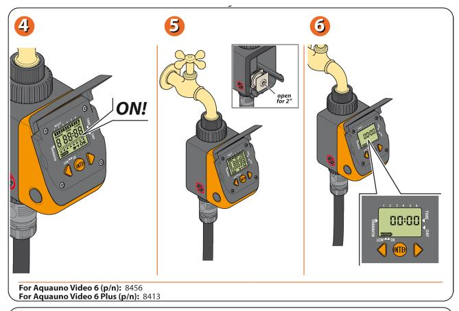
Pressing the ENTER key button, the message OK will appear. Set the current time using the FORWARD/BACK key buttons. Keeping the FORWARD or BACK key buttons pressed, the numbers will scroll more quickly. Having set the time, press ENTER, and the message OK will appear.
