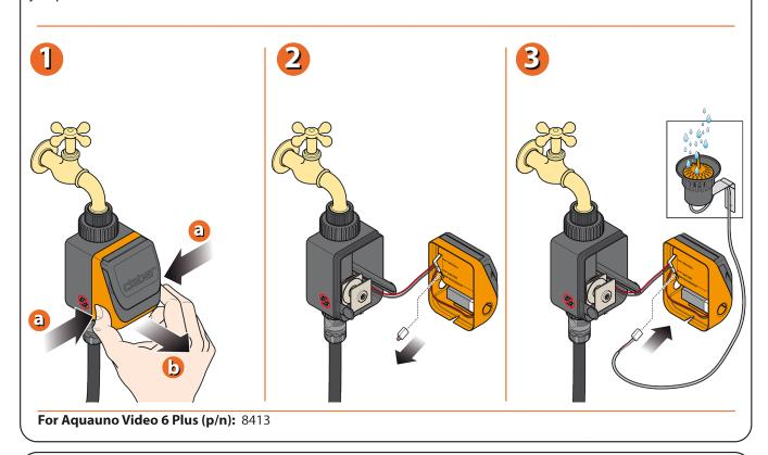
At the end of the warm season and before the first winter frosts, disconnect the timer from the tap and store it indoors, bearing in mind to remove the battery.
