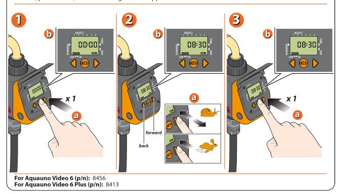
Programming is managed by way of pages presented in the display. Each page has two functions: view programme and, pressing ENTER, modify programme. Pressing FORWARD, the display will show the second programme of the line.
