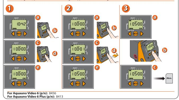
Press the FORWARD key button once. The display shows "1=progr. 1 CLOSED". The timer sets the 'close' time automatically one minute after the 'open' time (in the example: 05:01). Press ENTER to set the 'close' time, in the same way as for the 'open' time (e.g. 05:20). Set the required 'close' time using the FORWARD/BACK key buttons. The symbol for programme 1 continues to be displayed after the programme has been stored. Press ENTER to conclude the programming procedure.
