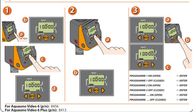
Suppose watering is to be programmed from the current time (e.g. 10:42). Press the FORWARD key button once. The display shows "1=progr.1 OPEN". The time appears as 00:00; press ENTER to set the opening time as required. The message OK means that the 'open' time can now be selected with the FORWARD/BACK key buttons. The symbol for programme 1 also appears at the top of the display. Having set the time (e.g. 5:00), press ENTER. The OK message disappears and the watering start time is saved.
