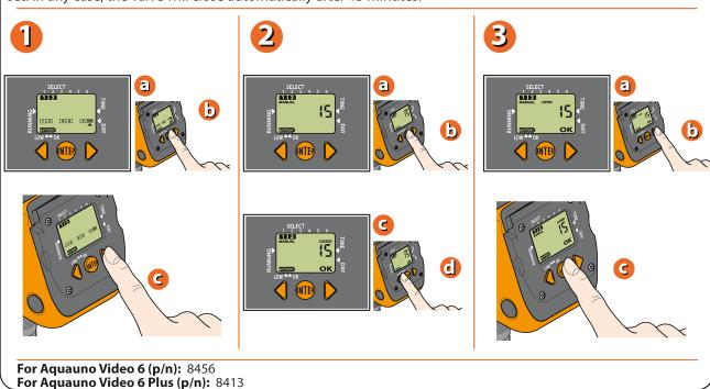
To delete a programme, press FORWARD until the display shows the "CLOSED" page of the programme to be removed. Press ENTER, then press the FORWARD / BACK key buttons simultaneously.
